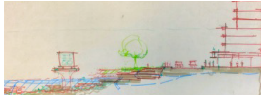
The CN Line as a trestle across Ambleside, with the natural shoreline right up to the south side of Marine Drive, meaning occasional flooding, allowed for by adaptive street surfaces. Density on the north side of Marine Drive is significantly increased, with ground level accommodation of storm surge events.
