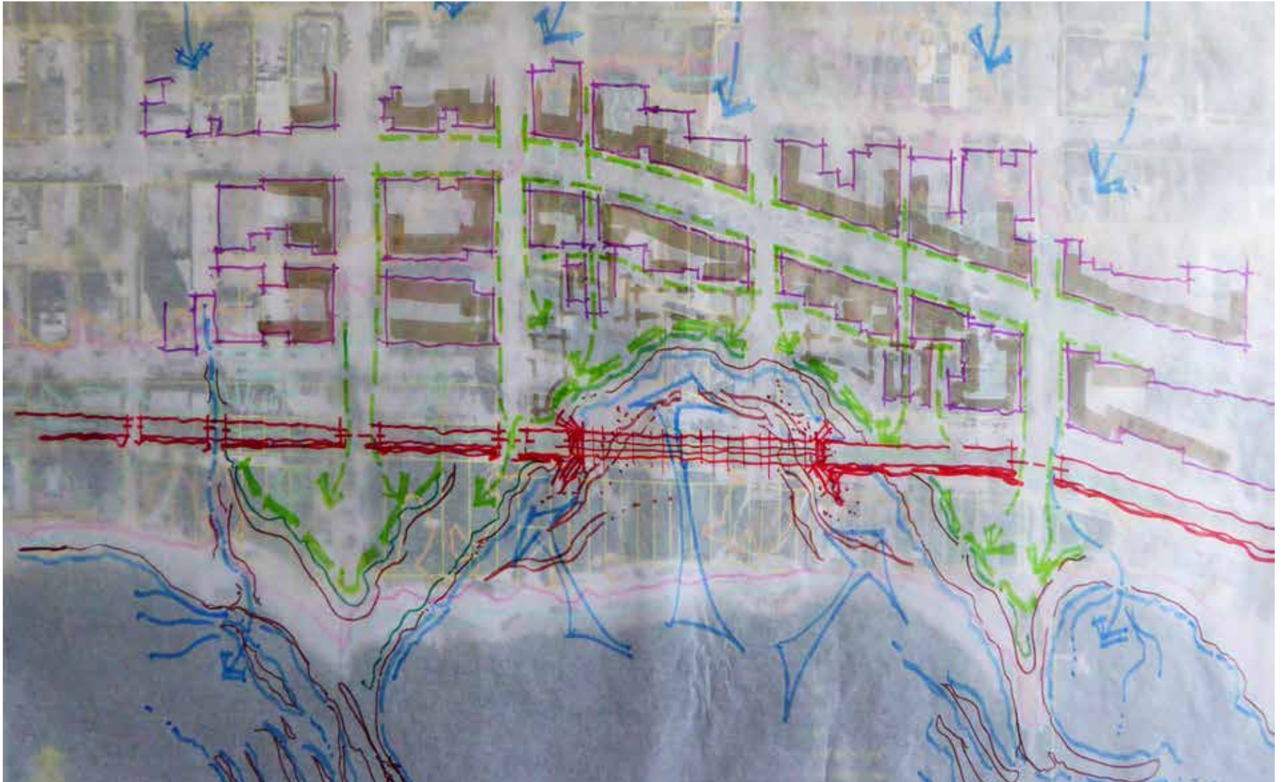
SCENARIO 2: THE HYBRID. The CN line as a raised-trestle, with some development pulled back as far as Marine Drive to accommodate rising sea levels on lower elevation lands. Restored and enhanced estuaries allow build-up of sediment and other materials over time which further buffers the area from storm surges.
