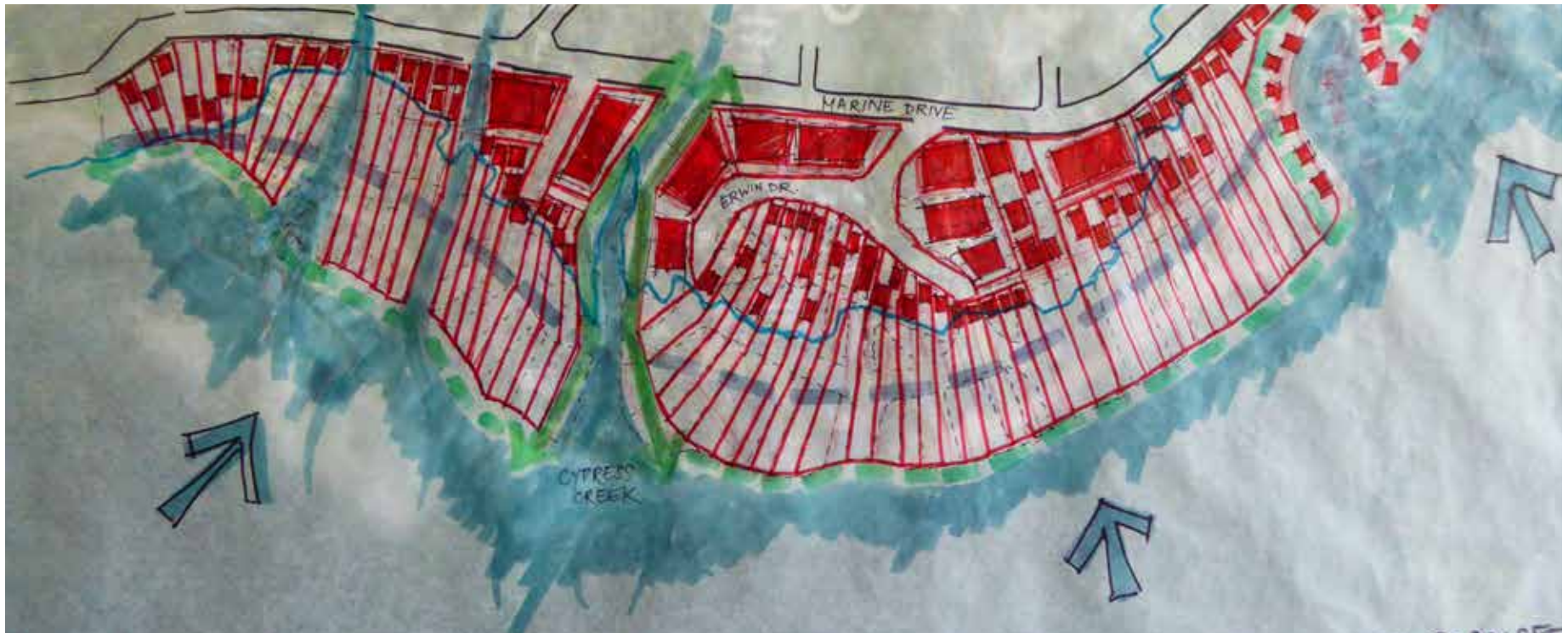
SCENARIO 2: THE SHARED WATERFRONT. Lot reconfiguration based on expected ingress of water with minimal protection. DFO site in the east is repurposed as a new pilot.
